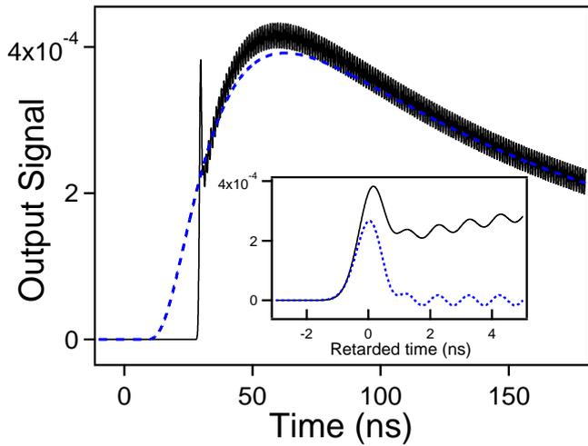
Figure 15: (Color online) Response to the canonical input signal for  $\sigma \approx 0.3 \text{ S/m}$  (other parameters as for the inset of Fig. 14). The solid (dashed) line is the exact numerical result (the analytical result obtained by considering the sole effects of conductivity). Inset: enlargement of the output signal around  $t = t_B$ . Here the dashed line is the analytical result derived from Eq. (48).
