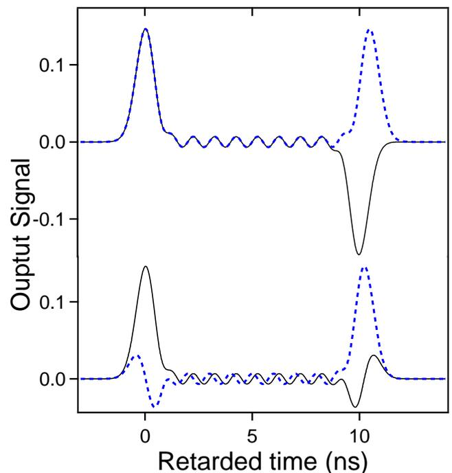
Figure 6: (Color online) Responses to input signals with a long rectangular envelope for  $\alpha_c \ell = 5$ . The upper curves are obtained for  $v(0, t) \propto \sin(\omega_c t)$  with  $T = 10 T_c$  (solid line) and  $T = 10.5 T_c$  (dashed line). The lower curves are obtained for  $T = 10.25 T_c$  with  $v(0, t) \propto \sin(\omega_c t)$  (solid line) and  $v(0, t) \propto \cos(\omega_c t)$  (dotted line). Note that, in the latter case, the postcursor can completely dominate the precursor.
