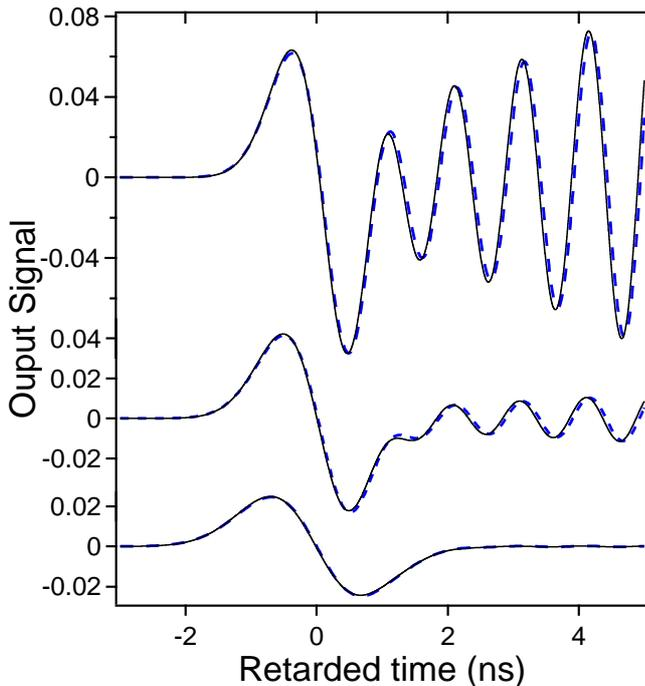
Figure 8: (Color online) Responses to the input signal  $(t/T_r)u_H(t)\sin(\omega_c t)$  normalized to  $1/(\omega_c T_r)$  for  $\alpha_c \ell = 6, 8,$  and  $12$  (from top to bottom). The solid (dashed) line is the FFT exact solution (the approximate analytical solution in terms of error functions).
