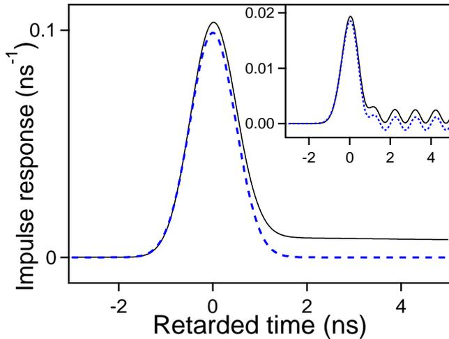
Figure 14: (Color online) Impulse response of water for  $\ell = 1$  m ( $t_B \approx 29.6$  ns) and  $\sigma \approx 0.1$  S/m. The solid (dashed) line is the exact numerical result (our approximate analytical result). Inset: corresponding response to the canonical input signal  $u_H(t) \sin(\omega_c t)$  with  $\omega_c = 2\pi \times 10^9$  s $^{-1}$ .
