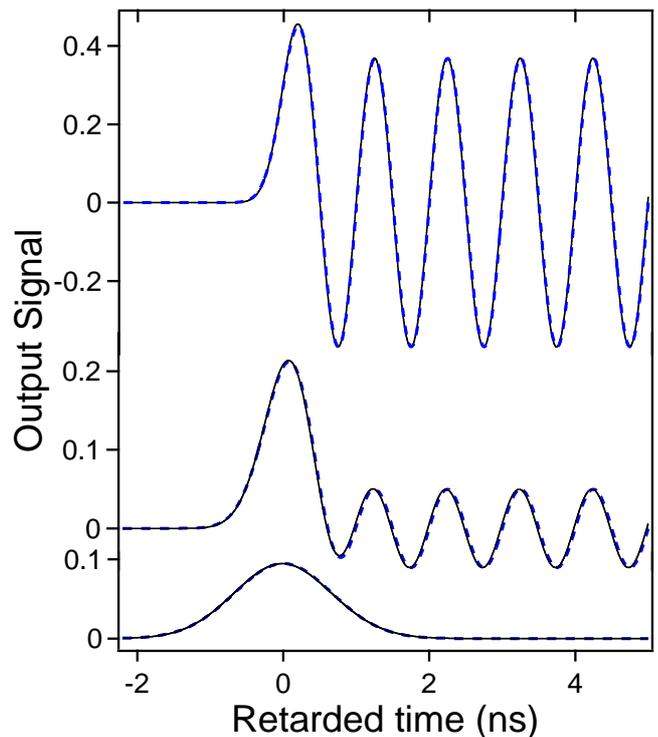
Figure 2: (Color online) Responses to the input signal  $u_H(t) \sin(\omega_c t)$  as a function of the time retarded by  $t_B$ , for  $\alpha_c \ell = 1, 3$  and  $10$  (from top to bottom). The solid (dashed) lines give the exact numerical solution (our analytical solution in terms of error functions). Note that for the carrier frequency considered ( $\omega_c / (2\pi) = 1 \text{ ns}^{-1}$ ), the optical thickness  $\alpha_c \ell = 1$  is attained for  $\ell = 21.6 \text{ cm}$ .
