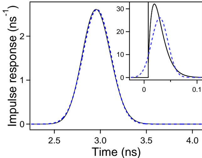
Figure 1: (Color online) Impulse response of deionized water as a function of time for a propagation distance  $\ell = 10$  cm leading to  $t_B = 2.96$  ns and  $\beta = 4.63$  ns $^{-1}$ . The solid [dashed] line is the exact numerical result obtained by FFT [the Gaussian shape given by Eq. (7)]. Inset: the same for  $\ell = 1$  mm, leading to  $t_B = 29.6$  ps and  $\beta = 46.3$  ns $^{-1}$ .
