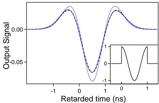
Figure 7: (Color online) Response to the input signal  $[u_H(t) - u_H(t - T_c)] \cos(\omega_ct)$  for  $\alpha_c\ell = 5$ . The solid, dashed and dotted lines are the exact FFT solution, the approximate analytical solution given Eq. (29), and the asymptotic solution given Eq. (26), respectively. Inset: input signal.
