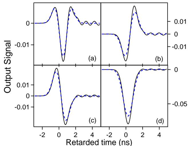
Figure 12: (Color online) Responses (solid line) to input signals with trapezoidal envelope of rise times  $T_r = T_c$  or  $T_c/2$  for  $\alpha_c \ell = 7$ . (a)  $T_r = T_c$ ,  $v(0, t) \propto \sin(\omega_c t)$ ; (b)  $T_r = T_c$ ,  $v(0, t) \propto \cos(\omega_c t)$ ; (c)  $T_r = T_c/2$ ,  $v(0, t) \propto \sin(\omega_c t)$ ; and (d)  $T_r = T_c/2$ ,  $v(0, t) \propto \cos(\omega_c t)$ . The asymptotic solutions (dashed lines) are given for comparison.
