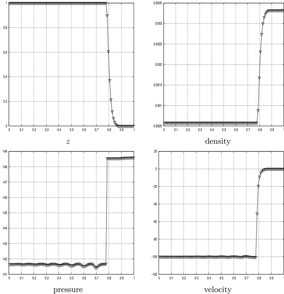
Figure 12:  $z$ , density, pressure and velocity profiles comparison for solutions obtained with the M-equilibrium scheme; the time step is given by CFL condition (37) (solid lines) and (38) ( $\nabla$  symbols).
