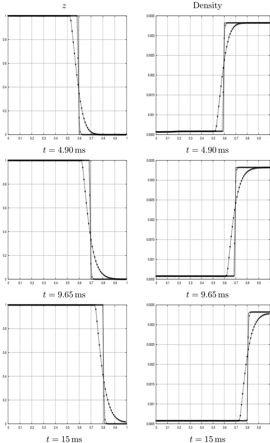
Figure 7:  $z$  and density profiles comparison between solutions for different mesh sizes obtained with the MT-equilibrium scheme; symbols  $\nabla$  and  $\times$  represent respectively solutions obtained with a domain discretize over 100 and 1000 cells while solid lines represent solutions obtained with a domain discretized over 5000 cells.
