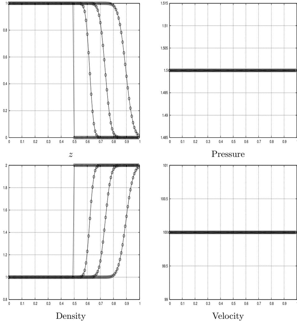
Figure 6: Time evolution of the MT-equilibrium solution computed with MT-scheme (dots) and the solution of the pure convective part of the system (15) computed with a Roe scheme (solid lines);  $t$  varies from  $t = 0$  s to  $t = 4$  ms.
