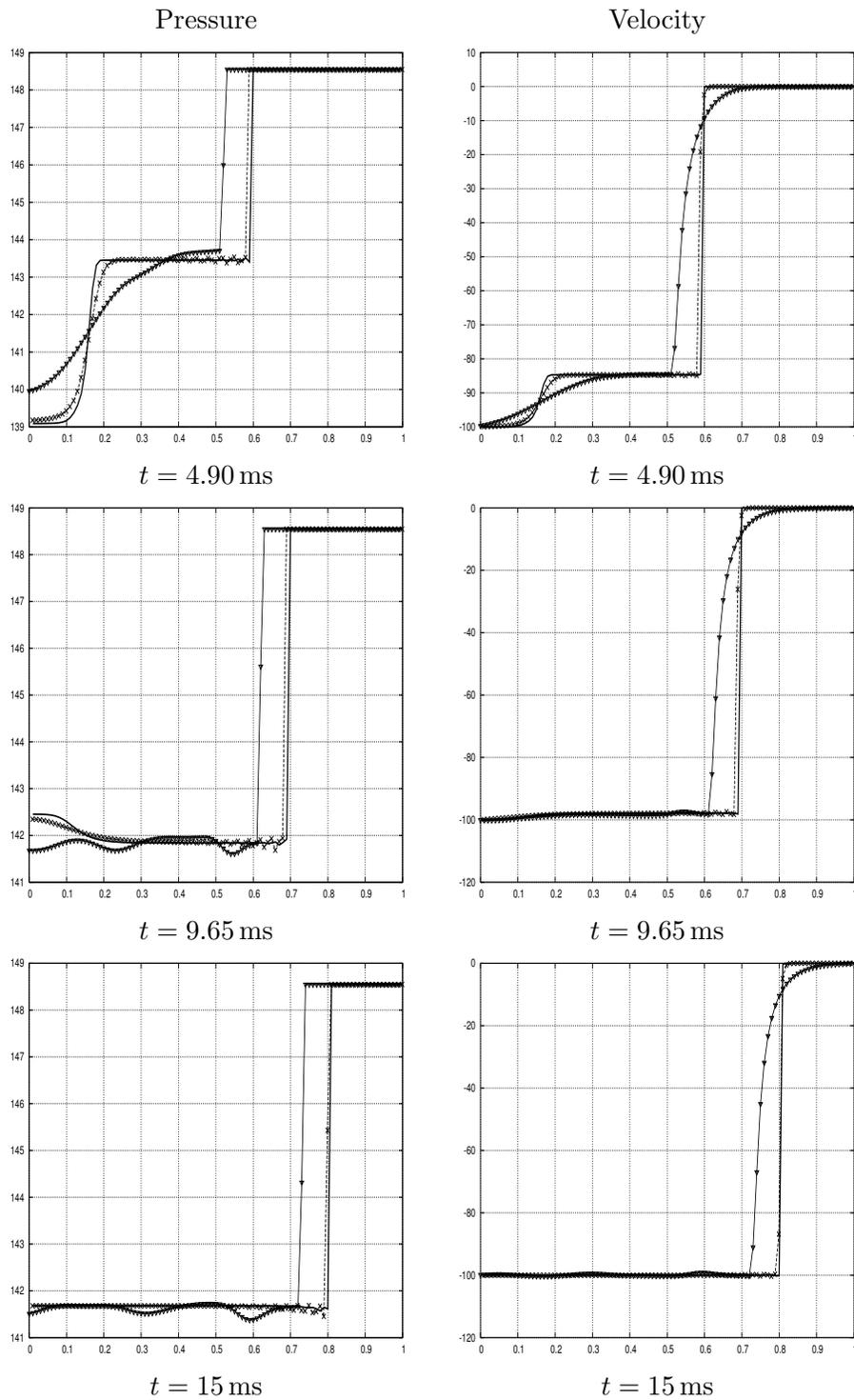
Figure 8: Pressure and velocity profiles comparison between solutions for different mesh sizes obtained with the MT-equilibrium; symbols  $\nabla$  and  $\times$  represent respectively solutions obtained with a domain discretize over 100 and 1000 cells while solid lines represent solutions obtained with a domain discretized over 5000 cells.
