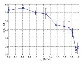
Fig. 16 Evolution of the aggregate volume wrt. the shear-stress.
