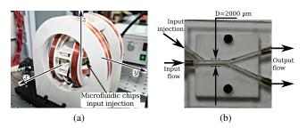
**Fig. 10** Experimental proof of concept setup: (a) 3D Maxwell-Helmholtz coils setup; and (b) Y-shaped microfluidic arterial bifurcation chip.
