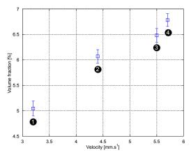
Fig. 14 Evolution of particle losses wrt. navigation speed.
