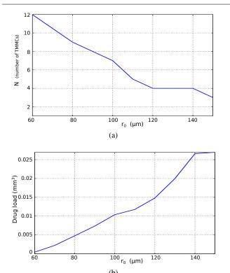
**Fig. 9** Evaluation of the optimum (a) number of microspheres for chain-like structures, and (b) the drug load capability as function of the TMMCs radius  $r_0$ .
