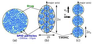
**Fig. 2** Magnetic microrobot: (a) single spherical TMMC, (b) ellipsoid-like aggregation and (c) chain-like agglomerate of TMMC.
