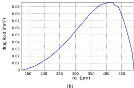
**Fig. 6** Evaluation of magnetization rate  $\tau_m$  (a) and drug load (b) as function of the radius for a magnetophoretic number  $C_{\rm mt}=1$  for spherical magnetic microrobots.
