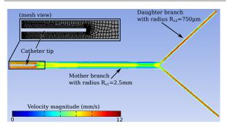
**Fig. 12** Computational fluid dynamics simulation of a microcatheter delivering bolus of aggregates of magnetic microparticles in a Y-shaped microfluidic channel. As shown, the parabolic profile of laminar flow prevails in the mother and daughter vessels.
