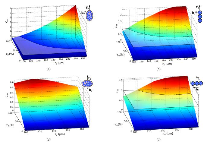
Fig. 7 Comparison of magnetophoretic number  $C_{\rm mt} = \mathbf{f}_{\rm m}/\mathbf{f}_{\rm d}$  for an ellipsoidal (a)–(c) and a chain-like (b)–(d) microrobots in parallel (a)–(b) and perpendicular (c)–(d) motions.
