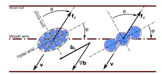
Fig. 3 Magnetic microrobot in vessel-like environment.
