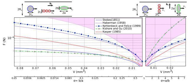
Fig. 4 Hydrodynamic drag forces  $\mathbf{f}_d$  for spherical, spheroid-like and chain-like superparamagnetic microrobots composed of TMMC aggregates as function of the bolus volume. The second abscissa shows the shape ratio  $\sigma = b/a = 1/N$  (left) and  $\sigma = a/b = N$  (right). Dimensions: TMMC radius  $r_0 = 100 \, \mu \text{m}$ , vessel radius  $R_v = 750 \, \mu \text{m}$ .
