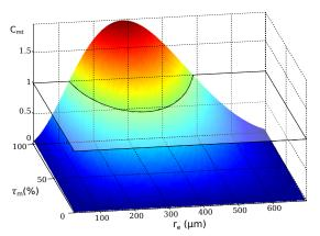
**Fig. 5** Magnetophoretic number  $C_{\mathrm{mt}} = \frac{\mathbf{f}_{\mathrm{m}}}{\mathbf{f}_{\mathrm{d}}}$  ratio as function of equivalent spherical radius  $r_e$  and magnetization rate  $\tau_m$  for spherical magnetic microrobots.
