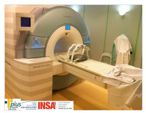
Fig. 18 The clinical Siemens Mangetom Verio 3T MRI scanner with the square acrylic box filled with water that contains bolus of aggregates.
