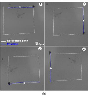
**Fig. 19** Navigation of a bolus of aggregates with a clinical MRI scanner: (a) artifact imaging from MRI data; (b) observed path with external digital microscope.
