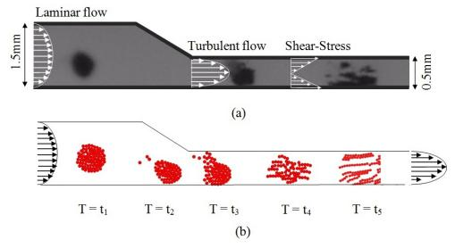
Fig. 17 Navigation of a bolus of aggregates in a daughter channel of radius  $750 \, \mu m$  toward a microfluidic vascular stenosis model of radius  $250 \, \mu m$ . (a) navigation of a magnetic bolus of radius  $r_0 = 250 \, \mu m$  in a stenosis vascular phantom and breaking in multiple clots due to shear-stresses; and (b) computational simulations using Discrete Particle Modeling software.
