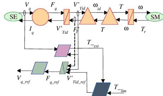
Fig. 9. Control structure for an active claw application.
