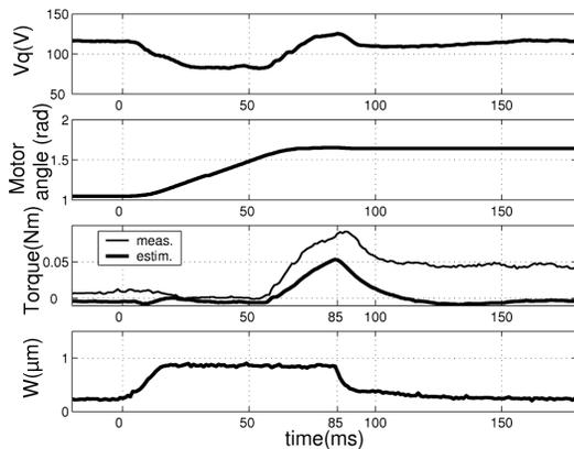
Fig. 11. Internal variables of the motor for a closing sequence of a TWUM actuated claw, with limitation of the torque.
