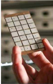
Figure 15: A manufactured tactile plate made up with 28 piezo cells glued onto the copper beryllium plate.
