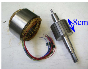
Figure 2. Experimental 5-phase motor.
