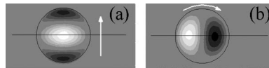
FIG. 10. Vorticity field obtained by artificially moving the LCD. (a) Effect of an upward translation. (b) Effect of a clockwise rotation.
