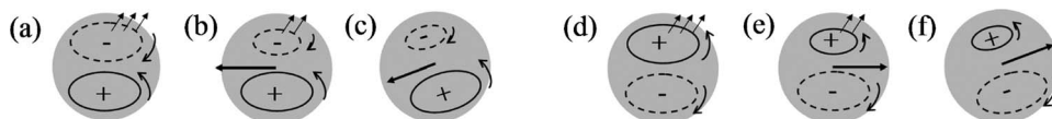
FIG. 15. Explanation of the rotation of the displacement mode in a vortex subjected to a localized action of viscosity shown by the arrays of arrows. The vortex is shown in grey and the loss of vorticity through the oval boundary by the array of arrows. The curved arrow indicates the rotation of the vorticity zones. The initially well-balanced vortex dipole of perturbation in (a) loses vorticity at the oval boundary. This results in frame (b) in a relative strengthening of the lower lobe compared to the upper one. This leads, through the term (\mathbf{u}' \cdot \nabla) \bar{\zeta} of Eq. (22), to the modification of the vortex position, initially in an upward position, such that the displacement mode rotates as shown in frame (c). The induced velocity \mathbf{u}' is shown by the arrow on the vortex. The case with the displacement mode the other way around in frames (d), (e), and (f) evolves in the same way.
