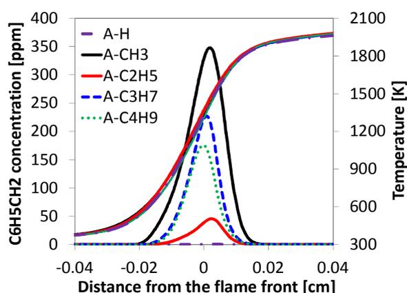
Figure 7: Concentration profiles of the  $C_6H_5CH_2$  radical in proximity of the flame front for the five fuels considered in our analysis. The symbol A-represents the phenyl group ( $C_6H_5-$ ). (For the benzene flame, the concentration of benzyl radical is negligible).
