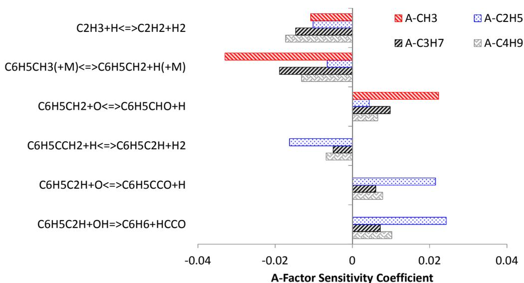
**Figure 6:** A-sensitivity factor analysis on the flame speed of four alkyl-benzenes: toluene, ethylbenzene, *n*-propylbenzene, *n*-butylbenzene using modified heat capacities for nitrogen.  $T_u = 358$ ,  $\Phi = 1$ , flame temperature is  $2337 \text{ K} \pm 1 \text{ K}$  for all the case. The symbol A-represents the phenyl group ( $\text{C}_6\text{H}_5-$ ).
