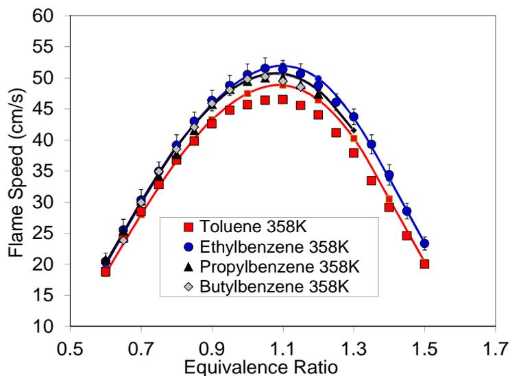
Figure 4: Comparison of laminar flame velocities (symbols: experiments, lines: calculations) as a function of equivalence ratio for alkyl-benzenes from toluene up to *n*-butyl-benzene at 358 K. Toluene data are from a previous study [12]. The lines for propyl-benzene and butyl-benzene overlap.
