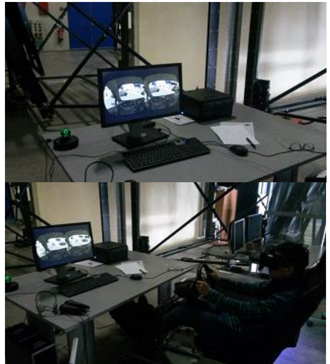
Fig. 1. Oculus rift HMD in driving simulation experiments
