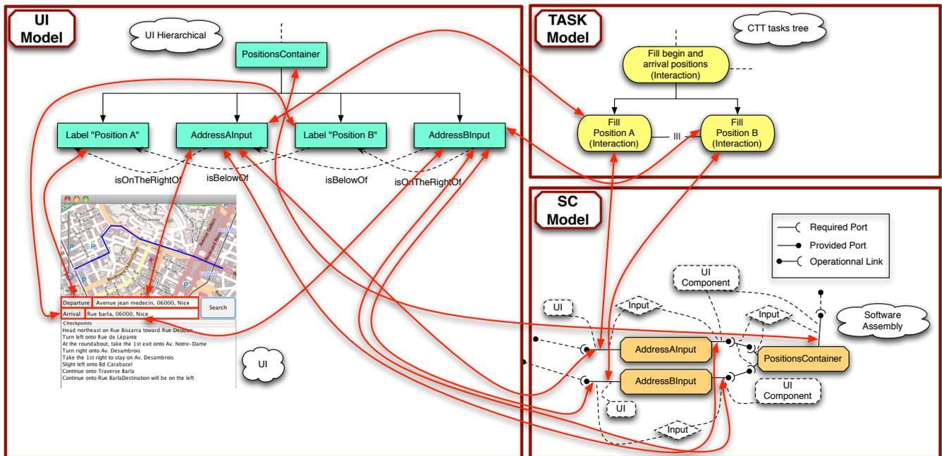
Figure 1: Excerpt of the application model linking UI, Tasks and Software Components (SC).
