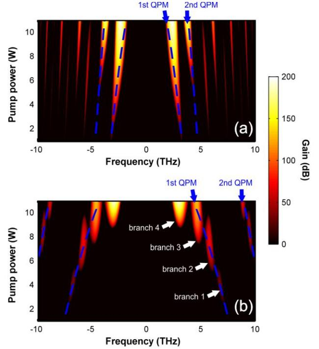
Fig. 1. Evolution of the output gain spectrum according to the input power for an average dispersion of  $0.7 \text{ ps}^2/\text{km}$  (a) and  $0.13 \text{ ps}^2/\text{km}$  (b). The corresponding pumping wavelengths are 1536 and 1554 nm. Results are obtained from the linear stability analysis based on the Floquet theory. The predictions from Eq. (3) are plotted with blue line.
