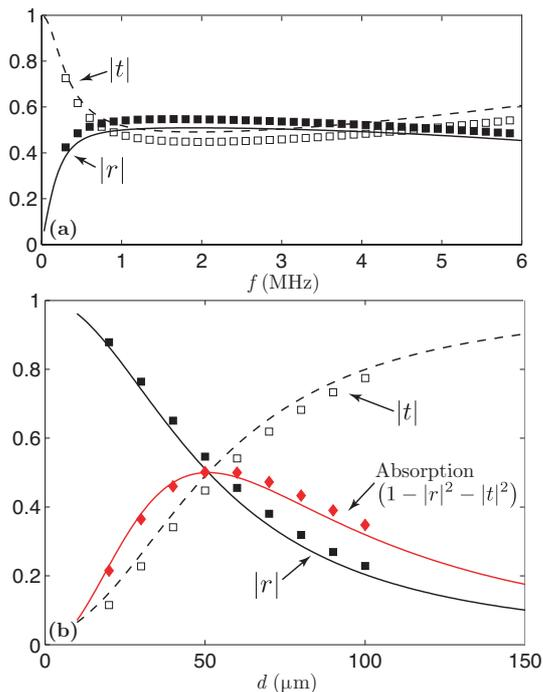
FIG. 2: (a) Transmission and reflection predicted by the model (lines) and finite element simulations (symbols) for  $\eta = \eta^*$ . (b)  $|t|$ ,  $|r|$  and absorption ( $A = 1 - |r|^2 - |t|^2$ ) at 2 MHz as a function of bubble spacing  $d$ .
