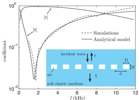
FIG. 1: Comparison between Eq. (1b) and simulation data extracted from figure 16 in Hladky-Henion et al. [20], for the transmission coefficient through a layer of air cylinders ( $H = 2$  cm,  $D = 1.5$  cm) on a square lattice ( $d = 5$  cm) in silicone.
