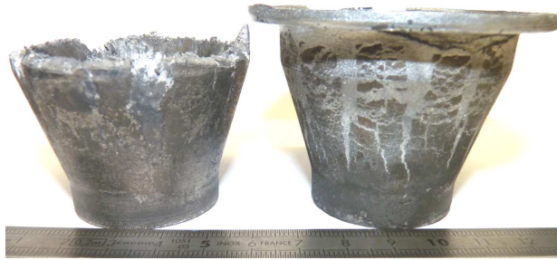
Fig.9 Parts thixoextruded at 590 °C and 620 °C
