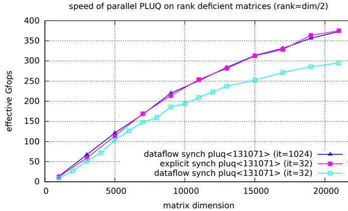
Figure 12: Performance of tile recursive PLUQ on 32 cores. Matrices rank is equal to half their dimensions. Note that the speed here ( $2/3 \times n^3/time$ ) does not correspond to the real number of operations when rank is less than the dimension.
