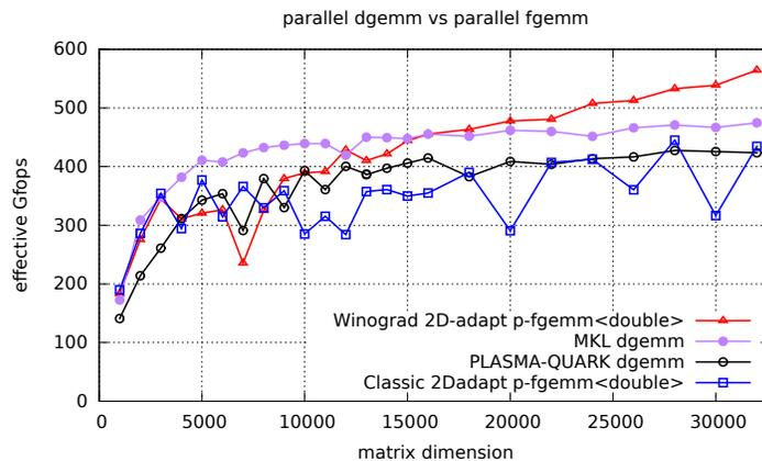
Figure 6: Speed of numerical matrix multiplication routines
