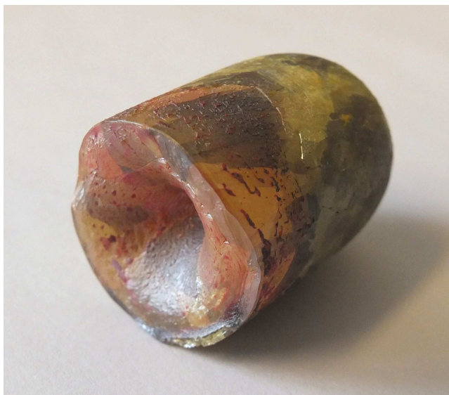
Figure 2: \text{AgGaGeS}_4 polycrystalline ingot after the first step : chemical synthesis.
