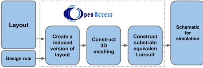
Fig. 2. The overall substrate extraction flow proposed.
