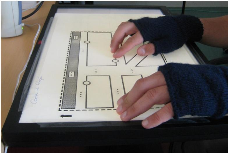
**Figure 1. Photograph of a user exploring an interactive map. The raised-line map overlay is attached on top of the touch screen. The user is wearing mittens to hinder unintended touch input from the palms.**
