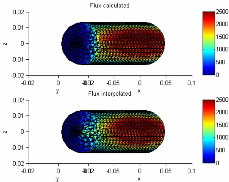
**Figure 4.** The intensity of the incident radiation on the outer surface of the preform (Visualized by Matlab): calculated (above) VS interpolated (below).
