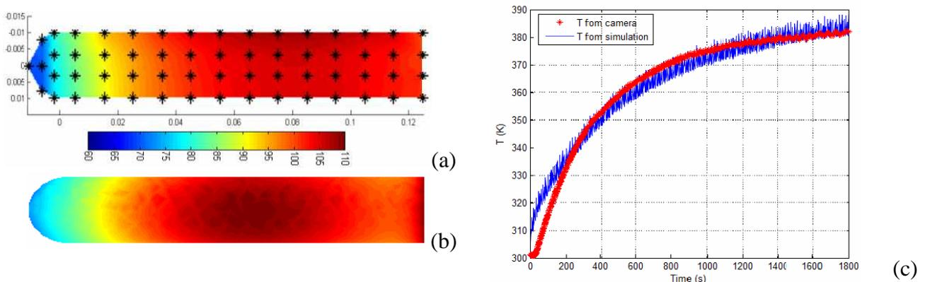
**Figure 5.** (a) Experimental results of the distribution of temperature on the outer surface of the preform at quasi steady state from thermal camera; (b) numerical results from Comsol; (c) evolution of the temperature on the center point of the outer surface
