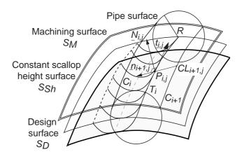
Figure 3: The geometry of constant scallop height tool path
