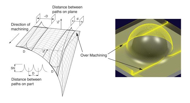
Figure 1: Tool paths tightening
