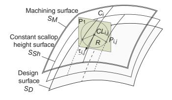
Figure 4: Discrete construction of the tool path
