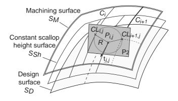
Figure 5: Discrete construction of the tool path
