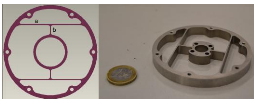
FIGURE 2. Rotary spring with variable stiffness
