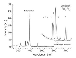
**Figure 4.** Excitation ( $\lambda_{em} = 612$  nm) and emission ( $\lambda_{ex} = 392.8$  nm) spectra for Eu-doped apatite-AEP colloids (spectra uncorrected for the spectral response of the apparatus), and background emission level due to the calcium phosphate matrix. AEP: 2-aminoethylphosphoric acid.
