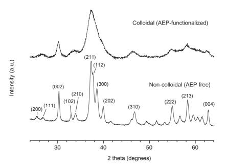
**Figure 1.** Typical XRD pattern for colloidal biomimetic apatite (AEP-functionalized, prepared at 100°C, and pH 9.5), and for a non-colloidal (AEP-free) counterpart with main XRD line indexation. XRD: X-ray diffraction; AEP: 2-aminoethylphosphoric acid.
