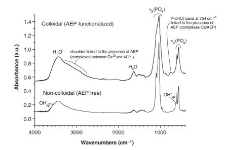
**Figure 2.** FTIR spectrum for colloidal biomimetic apatite (AEP-functionalized, prepared at 100°C and pH 9.5), and for a non-colloidal (AEP-free) counterpart. FTIR: Fourier-transform infrared; AEP: 2-aminoethylphosphoric acid.
