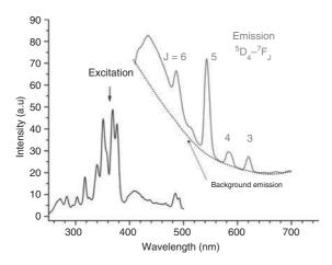
Figure 6. Excitation ( $\lambda_{em} = 540 \text{ nm}$ ) and emission ( $\lambda_{ex} = 379 \text{ nm}$ ) spectra for Tb-doped apatite-AEP colloids (spectra uncorrected for the spectral response of the apparatus), and background emission level due to the calcium phosphate matrix. AEP: 2-aminoethylphosphoric acid.
