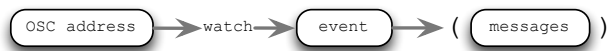
Figure 5. Basic mechanism to describe interactions: a set of messages is associated to an event by sending the watch message to an object.
