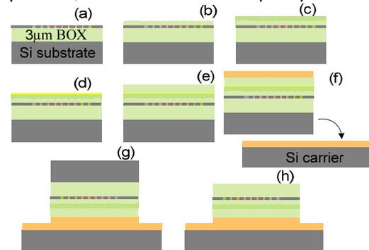
**Fig. 4:** Fabrication process of the grating coupler with bonded Al mirror. (a) Grating coupler fabrication based on standard e-beam lithography and ICP etching. (b)  $\text{SiO}_2$  deposition. (c) BPSG deposition and annealing. (d) Metallic mirror deposition. (e)  $\text{SiO}_2$  deposition. (f) BCB spinning for both sample and carrier wafer. (g) Bonding. (h) Si substrate removal.
