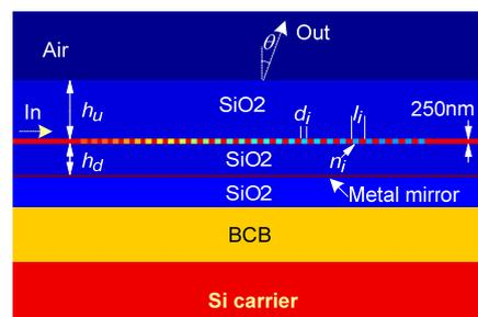
**Fig. 1:** Schematic structure of the proposed grating coupler.
