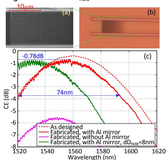
**Fig. 5:** (a) Scanning electron microscopy (SEM) image and (b) optical microscopy image of the fabricated grating coupler. (c) Measured coupling efficiency for the fabricated coupler with Al mirror with and without 8 nm hole size change, as well as for the same grating coupler fabricated on the same type of SOI wafer without Al mirror.
