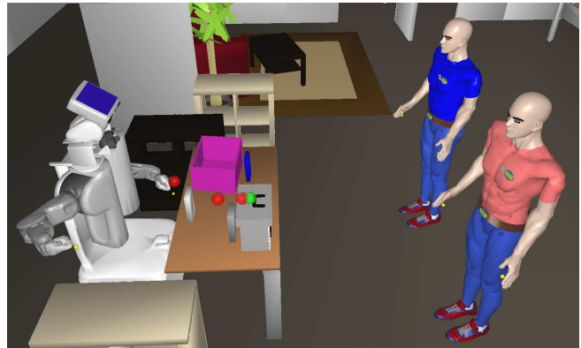
Fig. 1. Rendering of an environment as it is build and maintain by the system using SPARK data for furnitures, objects, humans and robot.
