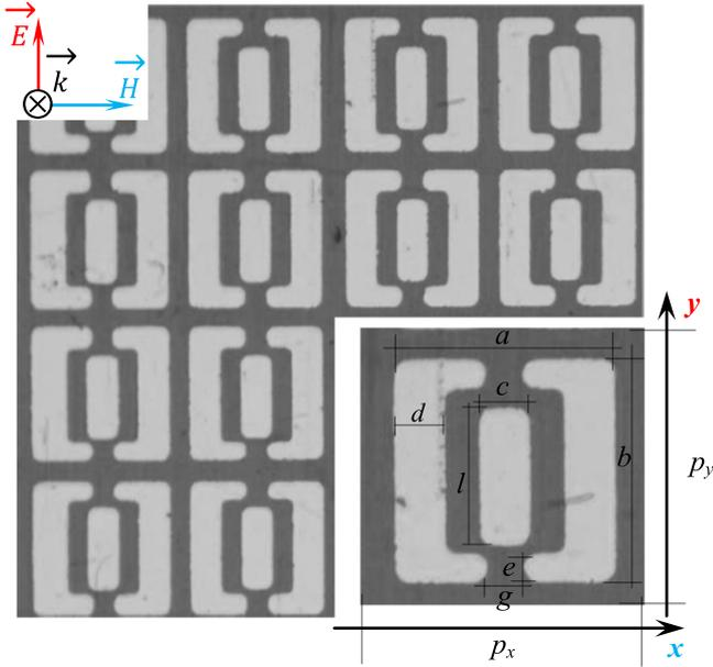
**Figure 1.** (a) Microscope image of the fabricated metamaterial with the relevant geometrical dimensions  $p_x=p_y=300\ \mu\text{m}$ ,  $a=b=250\ \mu\text{m}$ ,  $c=d=50\ \mu\text{m}$ ,  $e=20\ \mu\text{m}$ ,  $g=50\ \mu\text{m}$ ,  $l=150\ \mu\text{m}$ ,  $t_{\text{substrate}}=50\ \mu\text{m}$ .
