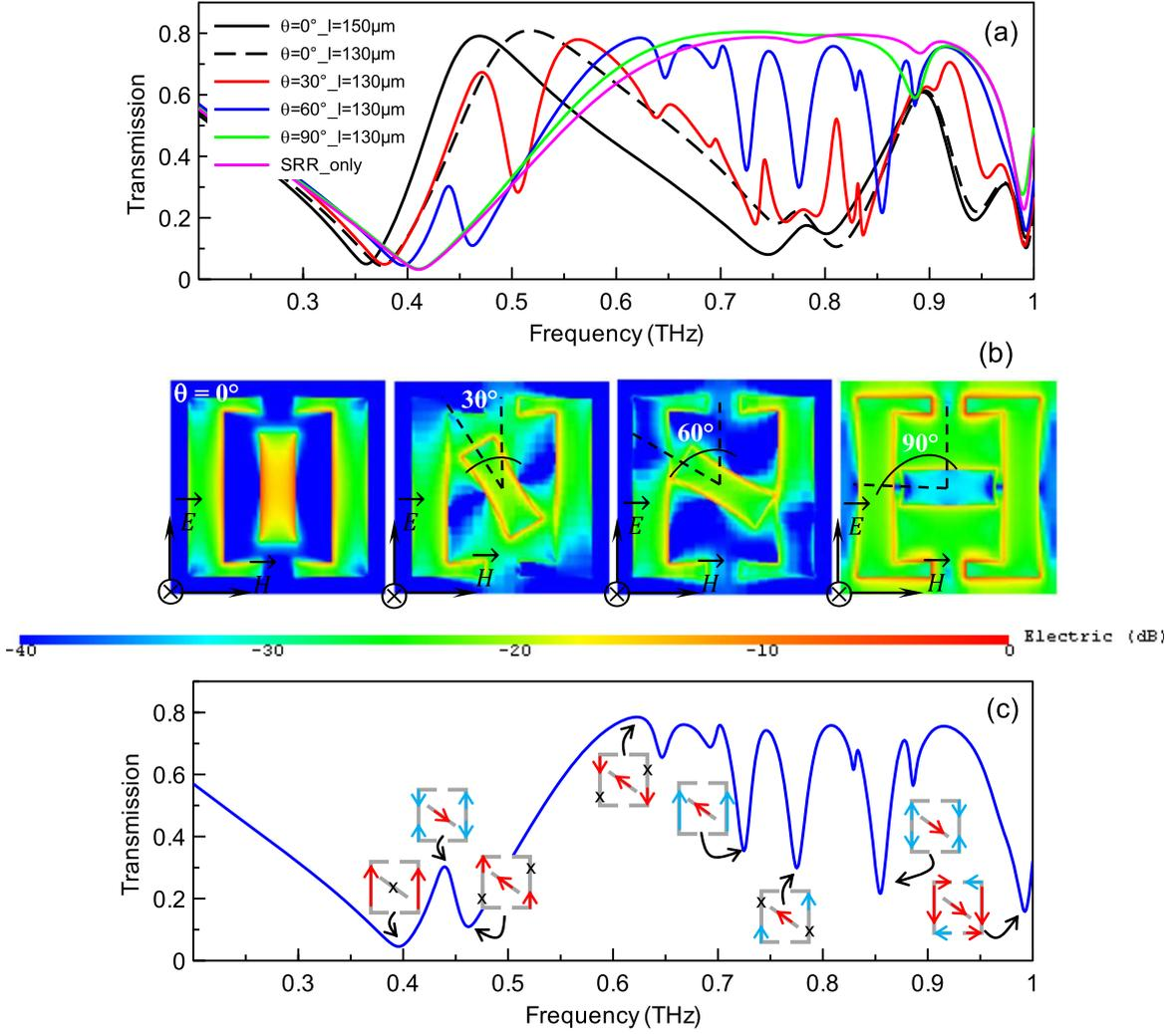
**Figure 5.** Evolution of the transmission spectra (a) and electric field distribution (b) around the first transmission peak at about 0.51 THz for different rotating angles  $\theta$  of the cut wires, with  $l = 130 \mu\text{m}$ . (c) Amplitude of the transmission for the sample with  $\theta = 60^\circ$ . The symbols represent the distribution of the surface currents in the SRR and the CW at each transmission dip and peak.
