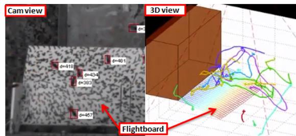
Figure 1: On the left, cropped top camera view of the flight board with detected flying bees. On the right, 3D reconstruction of the beehive with trajectories of bees being tracked at the entrance.
