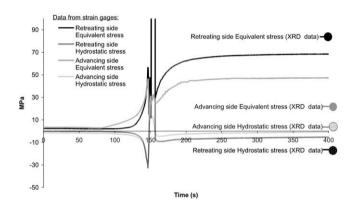
Fig. 10. Comparison between the stress evolutions during welding (strain gauges) and XRD results for FSW (1000 rpm, 200 mm min<sup>-1</sup>, tool 5 mm pin/13 mm shoulder).
