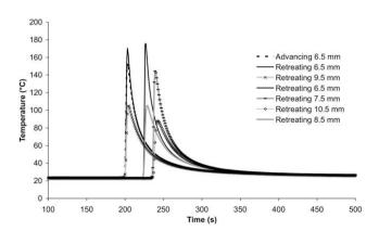
Fig. 9. Temperature measurements during FSW butt welding (600 rpm,  $2000 \text{ mm min}^{-1}$ ).
