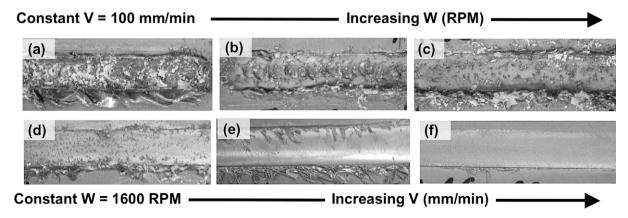
Fig. 4. Digital images of the superficial aspect of several "bead on plate" AZ31 welds: (a) W = 400 rpm,  $V = 100 \text{ mm min}^{-1}$ ; (b) W = 700 rpm,  $V = 100 \text{ mm min}^{-1}$ ; (c) W = 900 rpm,  $V = 100 \text{ mm min}^{-1}$ ; (d) W = 1600 rpm,  $V = 400 \text{ mm min}^{-1}$ ; (e) W = 1600 rpm,  $V = 600 \text{ mm min}^{-1}$ ; (f) W = 1600 rpm,  $V = 1000 \text{ mm min}^{-1}$ .
