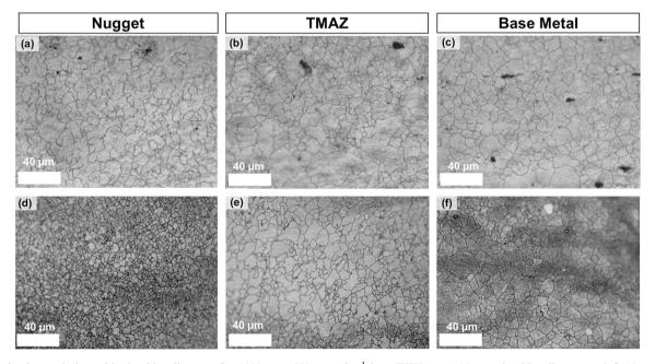
Fig. 7. Grain size evolution with shoulder diameter for 1000 rpm, 200 mm min<sup>-1</sup> butt FSW: (a-c) 13 mm shoulder diameter; (d-f) 10 mm shoulder diameter.
