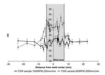
Fig. 11. Evolution of microhardness (0.98 N, 15 s) in FSW.
