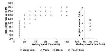
Fig. 3. AZ31 process window and defects observed.
