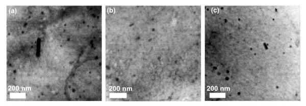
Fig. 8. Intragranular precipitation evolution in the butt weld nugget (tool 5 mm pin/10 mm shoulder): (a) (600 rpm, 2000 mm min<sup>-1</sup>); (b) (1000 rpm, 200 mm min<sup>-1</sup>); (c) base metal.
