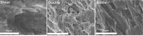
Fig. 13. Typical fractography of friction stir welds failure (1000 rpm, 200 mm min<sup>-1</sup>).
