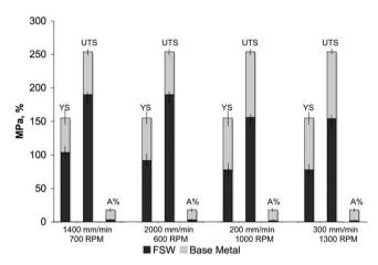
Fig. 12. Tensile properties of friction stir welds.
