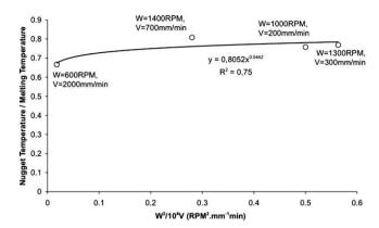
Fig. 15. Nugget temperature vs  $W^2/V$  ratio.
