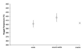
Fig. 16. Nugget temperature vs weld quality.
