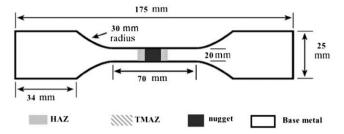
Fig. 2. Dumb-bell specimen specification.
