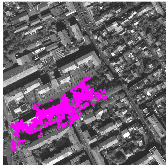
Fig. 4. Keypoints classified as change (example of Fig. 1).
