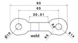
Fig. 2. Geometry of the specimen (dimensions in mm).
