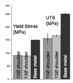
Fig. 3. Tensile properties of the FSW compared to base metal.
