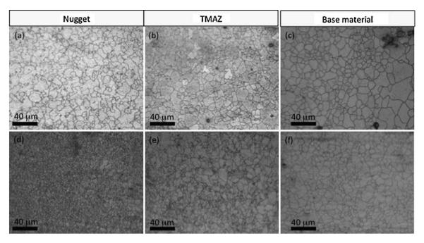
Fig. 7. Grain size evolution with shoulder diameter for 1000 rpm, 200 mm/min butt FSW (a-c) 13 mm shoulder diameter, (d-f) 10 mm shoulder diameter.
