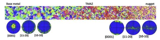
Fig. 8. EBSD analysis across the weld (10 mm shoulder diameter).
