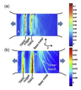
**Fig. 5.**  $\varepsilon_{22}$  Speckle deformation map of the sample top surface for (a) 10 mm shoulder diameter sample (F=4.5 kN) and (b) 13 mm shoulder diameter sample (F=3.5 kN), the A symbol indicates the advancing side location for each sample.
