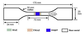
Fig. 1. Tensile specimen geometry.
