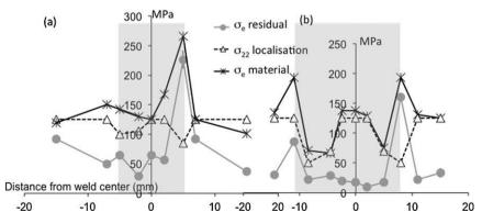
Fig. 6. Comparative evolution of the equivalent residual stress, localisation stress and equivalent material stress for (a) 10 mm shoulder diameter, (b) 13 mm shoulder diameter (the shaded area represents the weld zone).
