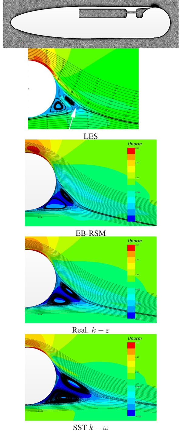
Figure 8: Velocity contours downstream of coanda airfoil at low injection Mach number ( $M_j = 0.39$ ) (Rumsey and Nishino, 2001).
