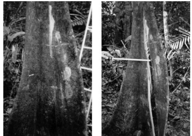
Fig. 7. Breakage observed during bending tests on the second Sloanea tree. The cracking buttress is lined up with the force direction and put in compression. Left, just after hearing the first crack; right, after increasing the load.
