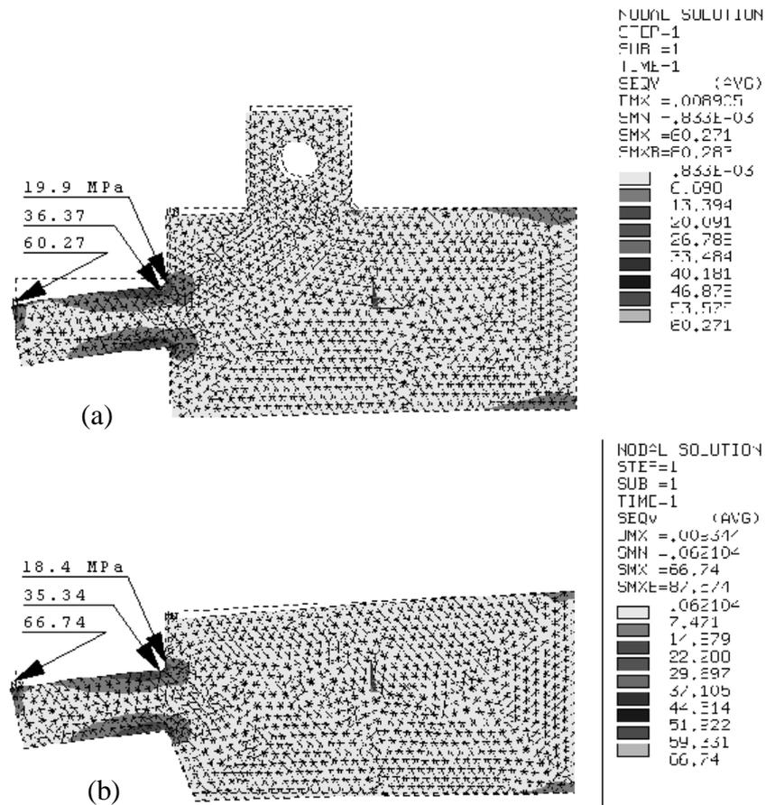
Figure 18 : Map of the Von-Mises stress criterion : (a) on the initial geometry, (b) on the simplified one, using the same calculation parameters in both cases.
