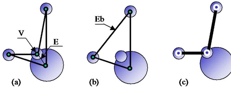
Figure 7 : Necessity of the edge collapse operator : (a) initial configuration, (b) result of the removal of the vertex  $V$ : the geometric restoration criterion is not satisfied for the boundary edge  $Eb$ , (c) result of the collapse process of the edge  $E$  : topological changes have occurred and the distance criterion is satisfied.
