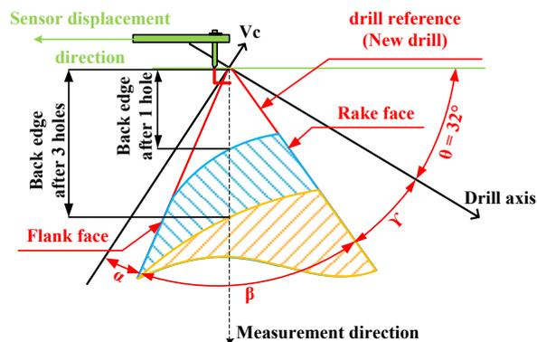
Fig. 7: Definition of the back edge criterion.
