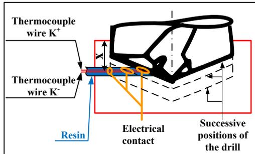
Fig. 2: Temperature measurement methodology.
