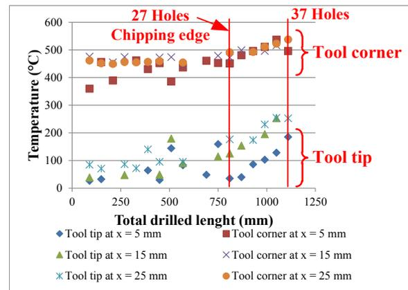
Fig. 9: Cutting temperatures evolution versus drilled length.
