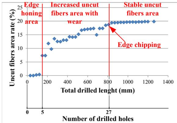
Fig. 11: Percentage of surface with uncut fibers.
