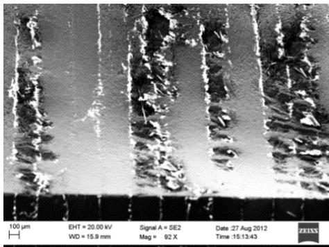
Fig. 16: Surface topography area of multidirectional CFRP T800M21.
