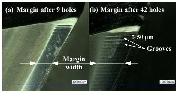
Fig. 6: Abrasive wear visible on the margin..
