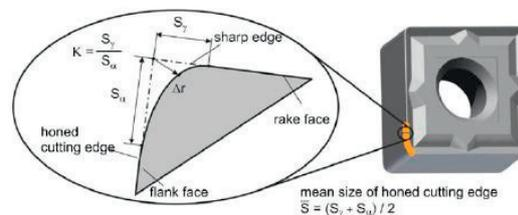
Fig. 1: Characterization of the cutting edge, after Denkena et al. [2]
