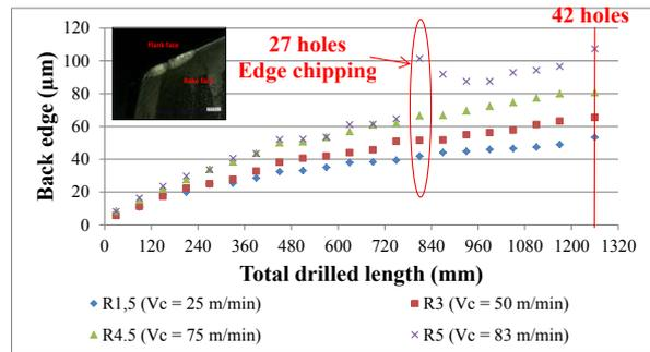
Fig. 8: Back edge criterion versus drilled length.
