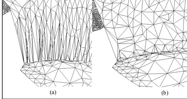
Figure 17: Influence of the 'equilateralization' process. (a) simplified polyhedron. (b) polyhedron simplified with an edge length criterion and obtained after the 'equilateralization' process.
