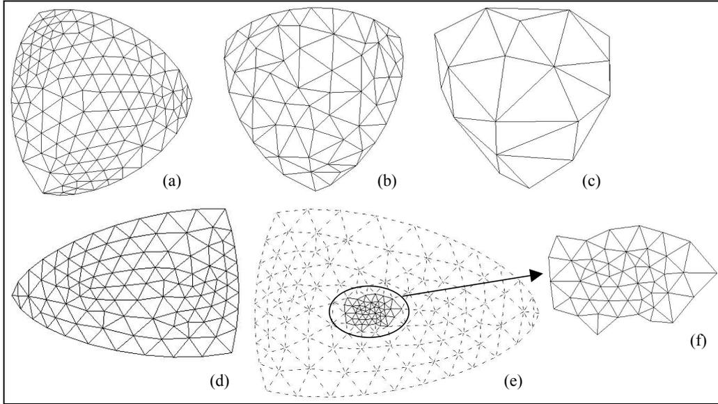
**Figure 6:** Various meshes of areas of spheres used for the computation of discrete mean curvatures using eq. (5) and eq. (6). (a) initial sphere of radius 1, (b) same sphere decimated with error zones of radius 0.01 (see section 4.1), (c) same sphere decimated with error zones of radius 0.05, (d) initial spherical area of radius 100, (e) initial spherical area after a mesh refinement operation, (f) subset of (e) where the enriched area has been extracted.
