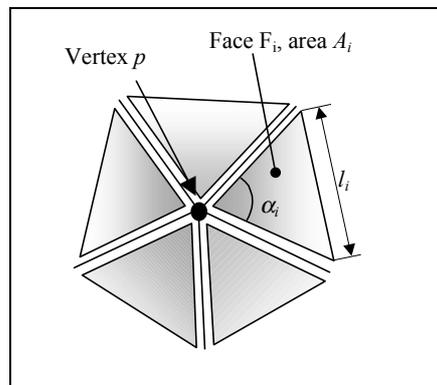
Figure 3: Geometric parameters of a star-set associated to a vertex  $p$ .
