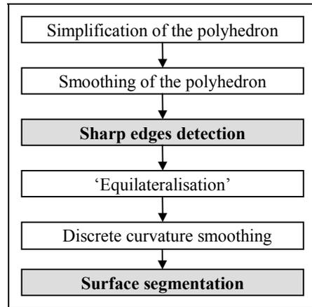
Figure 2: The main phases of the segmentation approach.
