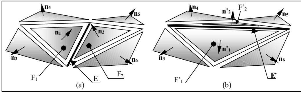
Figure 15: Parameters used by the  $Fm_a$  cost function before (a) and after (b) the edge swapping.
