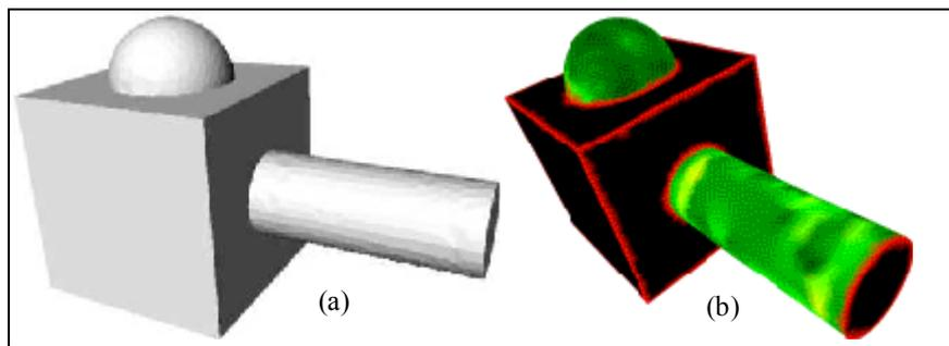
**Figure 9: (a) a polyhedron, (b) its map of the discrete absolute curvatures. The variation in the discrete absolute curvatures is due to the variations of the accuracy of the approximation errors and the irregularities over the mesh. Red areas indicate high curvature values, black ones designates areas where the discrete absolute curvature vanishes and greenish ones indicates intermediate values.**
