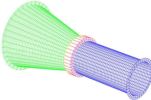
Figure 4: Mesh of the studied 3D assembly
