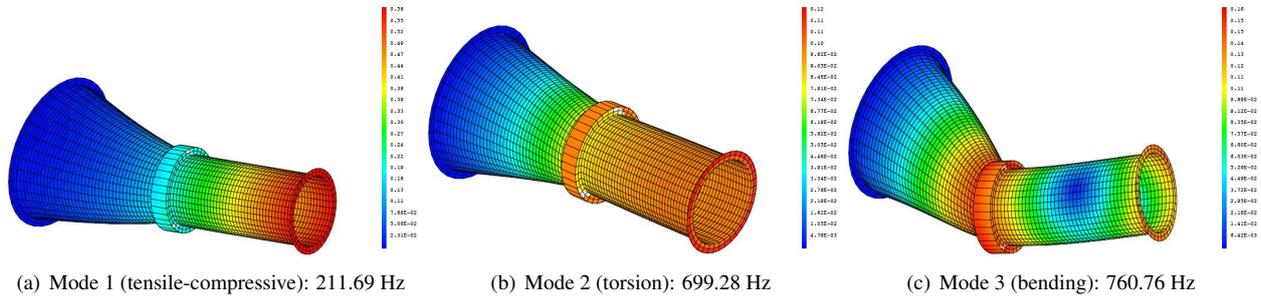
Figure 5: The shapes of the first three eigenmodes of the deterministic 3D assembly
