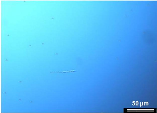
Fig. 1. Surface morphology of Ge doped layer grown on 8° off axis seed using 0.02 sccm GeH<sub>4</sub> flow at 1550 °C with C/Si ratio of 5 and 2.3 μm/h growth rate for 1 hour
