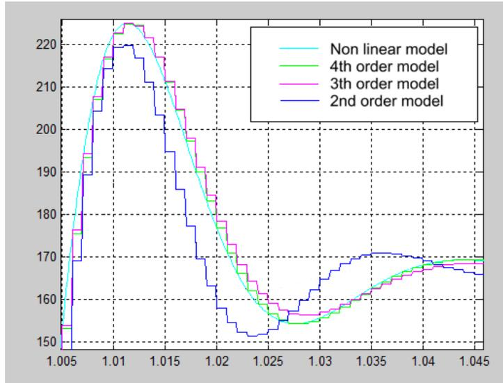
Figure 4; Step response of nonlinear and identified models.
