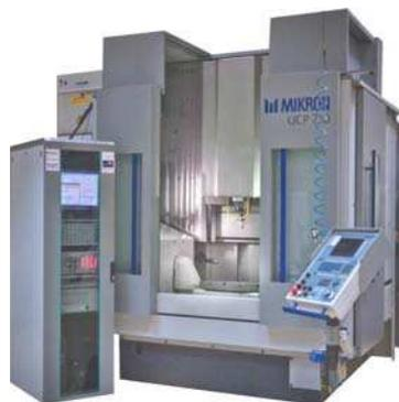
*Figure 1; Five-axis CNC Mikron machine.*
