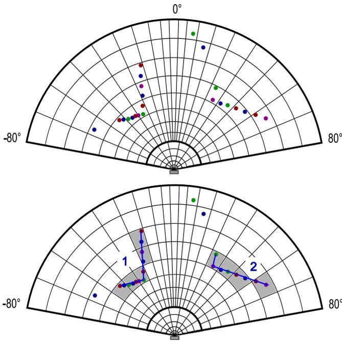
Fig. 3. Schematic grid design (not to scale) and segmentation procedure. Top: Projection of all scan points onto the grid. Bottom: Marking of grid cells with no. of points  $\geq$  threshold, connecting of adjacent grid cells and labeling.
