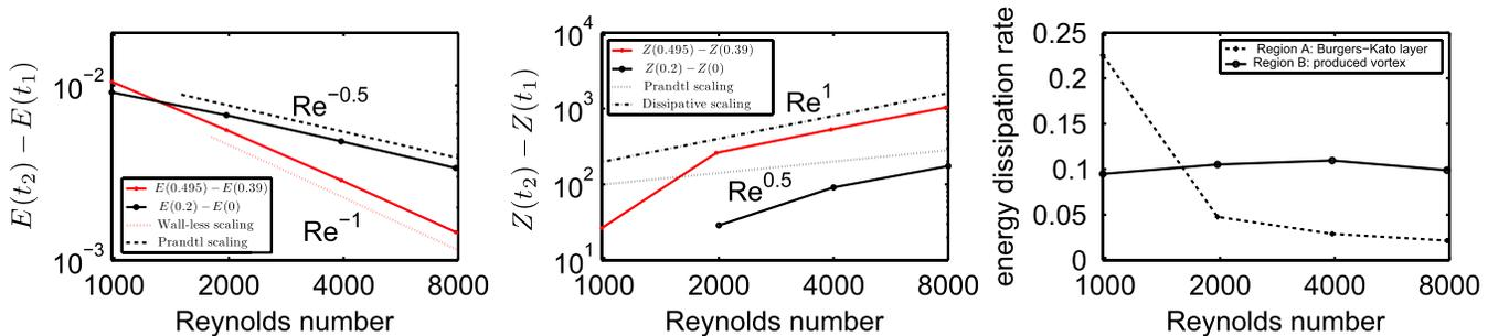
FIG. 3 (color online). Left and middle: Energy dissipation (respectively, enstrophy increase) as a function of  $Re$  for  $t \in [0, 0.2]$  and  $t \in [0.39, 0.495]$ . Right: Instantaneous energy dissipation as a function of  $Re$  at  $t = 0.495$  in regions A and B (see text).
