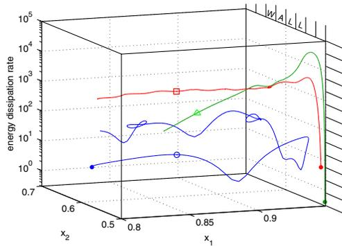
FIG. 4 (color online). Energy dissipation rate  $\nu|\nabla\mathbf{u}(x_1(t), x_2(t), t)|^2$  versus particle position  $[x_1(t), x_2(t)]$  for  $t \in [0.3, 0.495]$  along three Lagrangian trajectories, at  $\text{Re} = 3940$ . The full circles indicate the positions at  $t = 0.3$ . The hollow circle, square, and triangle mark the blue, red, and green trajectories, respectively.
