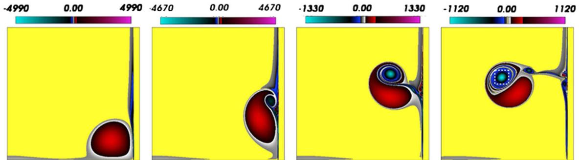
FIG. 1 (color online). Vorticity in the subdomain  $[0.708, 0.962] \times [0.5, 0.754]$  at  $t = 0.36, 0.4, 0.45$ , and  $0.495$  (left to right) for  $\text{Re} = 7880$ . The white dotted box at  $t = 0.495$  frames region  $B$  (see text). Black pixels correspond to  $\omega = \pm 300$  in all pictures.
