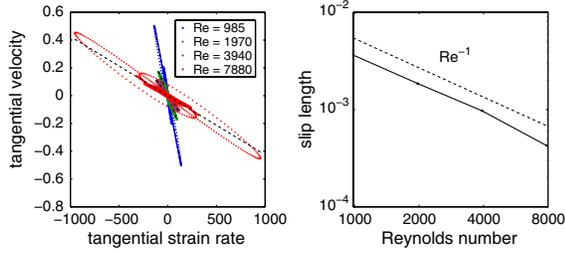
FIG. 2 (color online). Left: Tangential velocity  $u_2$  versus tangential strain rate  $\partial_1 u_2$ . The dashed lines are least squares linear fits. Right: Slip length  $\alpha$  defined by (6) as a function of  $Re$ .
