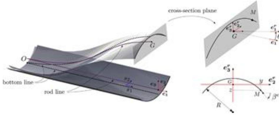
Fig. 2. Geometric and kinematic description of the tape spring (left) and its cross-section (right), with  $\delta_0; e_1; e_2; e_3$  the fixed orthonormal frame and  $\delta^r; e_1^r; e_2^r; e_3^r$  the rotated frame that follows the cross-section plane.
