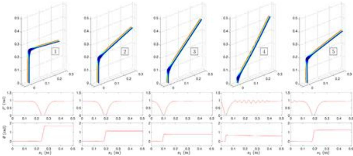
Fig. 12. Reconstructed deformed shapes of the tape at five significant time values during the deployment step for test (b), with superimposed color plots of angle  $b$ . From 1 to 5:  $t=0, 0.06, 0.085, 0.102$  and  $0.16$  s. Bottom plots: opening angle  $b^\delta$  and rotation  $h\delta_1$  of the cross-section plane along the rod for the five deformed shapes.
