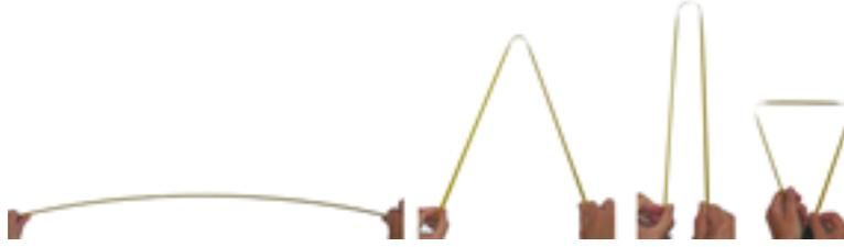
Fig. 1. Folding of a tape spring.
