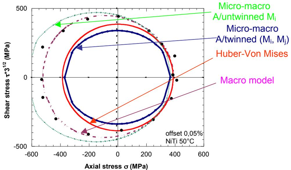
Figure 3 : Tension(compression)-torsion test on tubular sample , isotropic Ni-Ti
