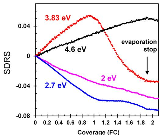
FIG. 2. (Color online) Evolution of the SDR signal for polarization along the NRs ( $[1\bar{1}0]$  direction) as a function of the Si coverage, at four energies of light: 2 eV (purple), 2.7 eV (blue), 3.83 eV (red), and 4.6 eV (black).
