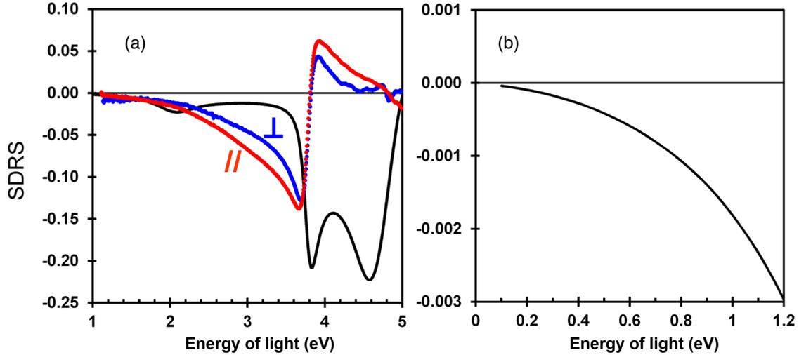
FIG. 3. (Color online) (a) Surface differential reflectance spectra measured for 1 Si FC on Ag(110). Red: light polarization along  $[1\bar{1}0]$ ; blue: light polarization perpendicular to  $[1\bar{1}0]$ . The black line is the calculation using the dielectric function of silicene, from Ref. [16]. (b) Zoom of the calculated SDR spectrum in the low-energy range.
