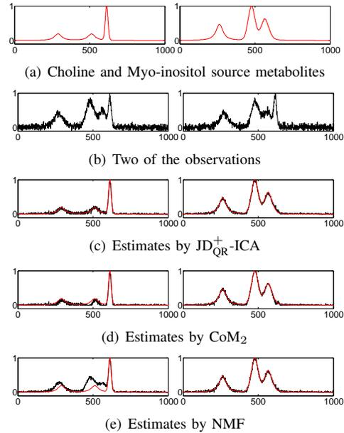
Fig. 3. MRS source metabolites, observations and estimated metabolites by  $\text{JD}_{\text{QR}}^+$ -ICA,  $\text{CoM}_2$  and NMF with SNR = 10 dB for one typical realization. The overlapping red lines in figures (c), (d) and (e) indicate the correct sources.
