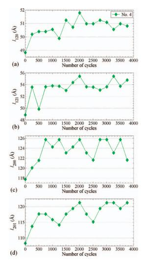
FIG. 6. — Evolution of the size of the crystallites during fatigue test 4 in the directions normal to the diffraction planes (120), (121), (200), and (201).
