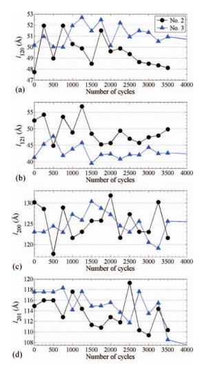
FIG. 5. — Evolution of the size of the crystallites during fatigue tests 2 and 3 in the directions normal to the diffraction planes (120), (121), (200), and (201).
