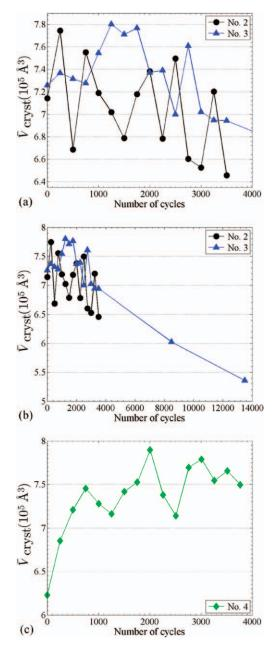
FIG. 7. — Evolution of the index of the volume of the crystallites (a) during the first 4000 cycles of fatigue tests 2 and 3; (b) during the first 13 500 cycles of fatigue test 3; and (c) during the first 4000 cycles of fatigue test 4.
