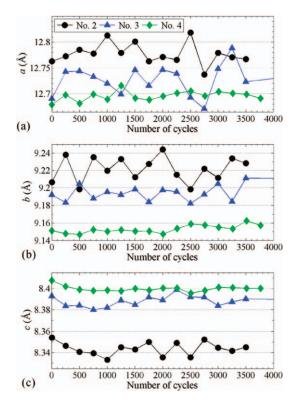
FIG. 9. — Evolution of the lattice parameters a, b, and c during fatigue tests 2 to 4.
