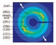
FIG. 3. — Example of diffraction pattern of crystallized NR in uniaxial tension. The white arrows show the tension direction. The Miller indices of the diffraction planes corresponding to the different reflections are indicated in the figure.
