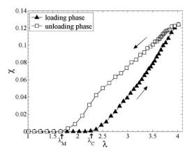
FIG. 2. — Evolution of the index of crystallinity during a quasi-static tensile test.
