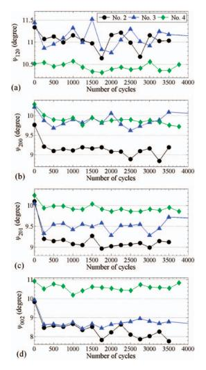
FIG. 8. — Evolution of the misorientation of the crystallites during the first 4000 cycles of fatigue tests 2 to 4.
