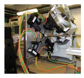
FIG. 1. — Fatigue-testing machine in DiffAbs beamline in synchrotron Soleil.
