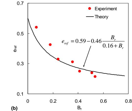
Figure 1. Particle crushing effect: (a) Evolution of breakage index versus modified plastic work, and (b) Evolution of reference critical state void ratio versus breakage index
