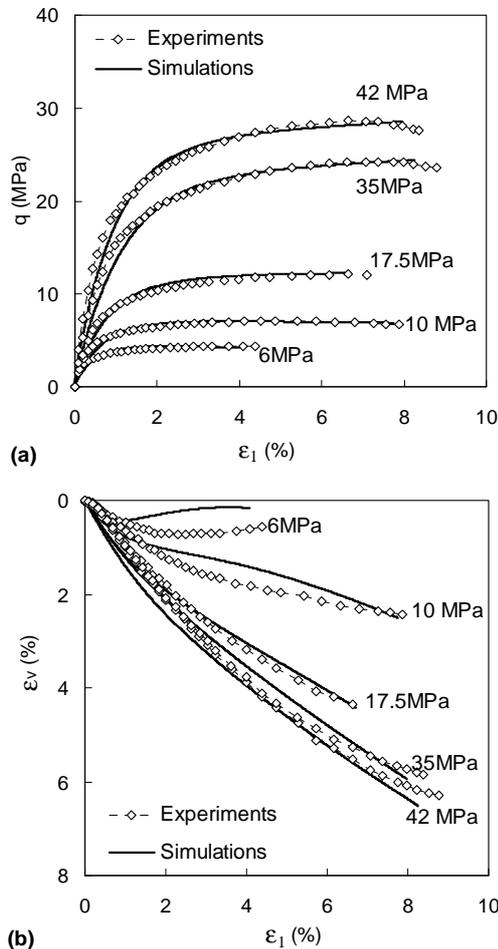
Figure 4. Comparisons between experimental results and simulations for drained triaxial extension tests: (a) deviatoric stress versus major principle strain, and (b) volumetric strain versus major principle strain
