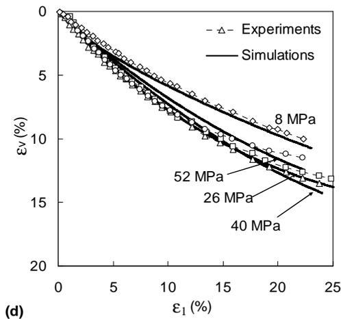
Figure 3. Comparisons between experimental data and simulations for drained triaxial compression tests: (a-c) deviatoric stress versus major principle strain; (b-d) volumetric strain versus major principle strain
