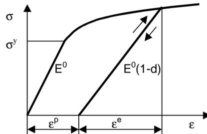
*Fig. 1: Theoretical inelastic stress/strain response of damaged composite*
