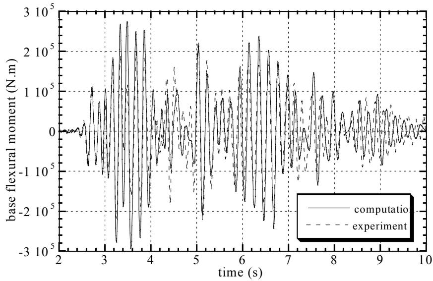
Figure 5: In plane flexural moment at the base : 0.15 g accelerogram
