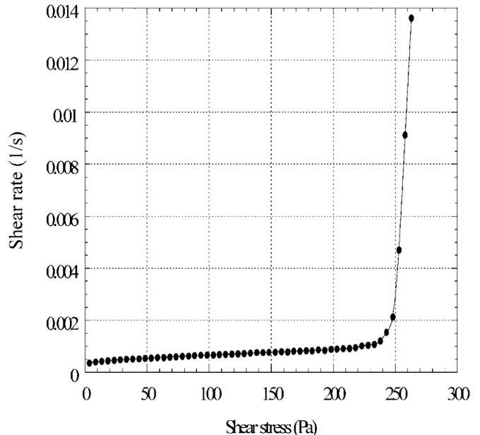
**Fig. 1** Evolution of the shear rate as a function of shear stress. The yield stress  $\sigma_y$  is the stress for which there is a significant increase of the shear rate. In this case  $\sigma_y \approx 250$  Pa
