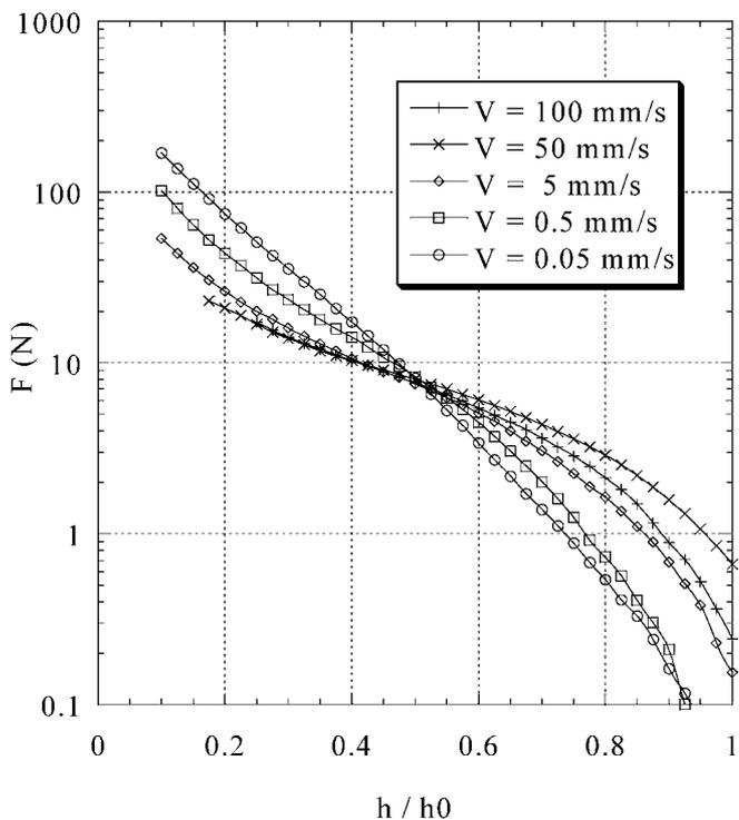
Fig. 3 Squeezing force vs normalized disc separation
