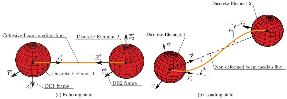
FIGURE 4: Cohesive beam bond configuration
