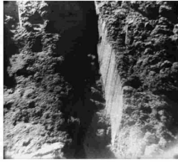
(a) Trench excavated by Surveyor 7 Spacecraft in Lunar subsurface soil (adapted from Perko et al., 2001).
