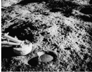
(b) The footprint of Spacecraft Surveyor 3 –Apollo 12 (adapted from NASA Image ID number: AS12-H-48-7110).
